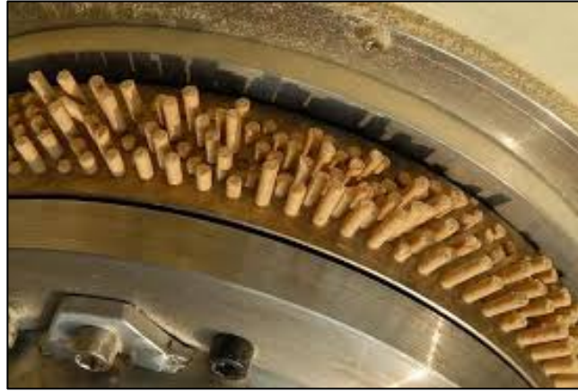
Figure 3.1: Wood pellet were produced from pelletizer.
